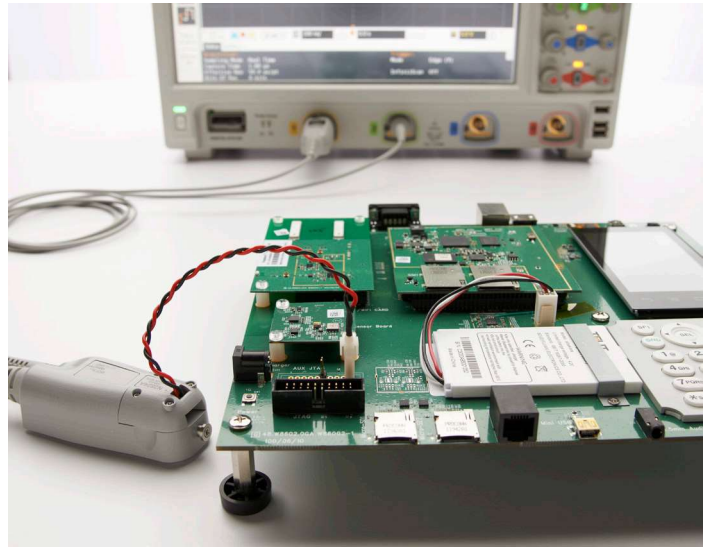
Figure 1. Keysight's ultra sensitive N2820A/N2821A current probes excel at measuring small current levels typically found in battery powered devices.
