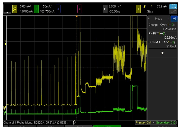
Figure 6. The InfiniiVision 3000 X- or 4000 X-Series oscilloscope can also be paired with the N2820A/21A current probes to provide the same simultaneous low- and/or high-gain views for wider dynamic range current measurement.
